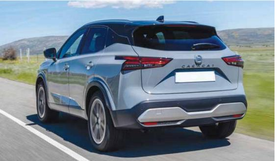
Riding on the Renault-Nissan-Missahi Alliance's latest Common Module Family (CMF) C-platform, the new Qashqai employs more lightweight material than before. The rear hatch, for instance, is fashioned from a composite material. The crossover employs an updated McPherson strut suspension set-up, with the rear suspension featuring a torsion beam on front-driven models and a multilink configuration on all-wheel-drive derivatives with 20-inch wheels.
