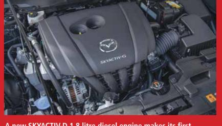
A new SKYACTIV-D 1.8 litre diesel engine makes its first appearance in the new Mazda CX-3, offering drivers both enhanced responsiveness and improved emissions performance. Two SKYACTIV-G 2.0 litre petrol engines now feature the innovations first adopted in the current Mazda CX-5, including edge-cut piston heads and high-dispersion injectors.
